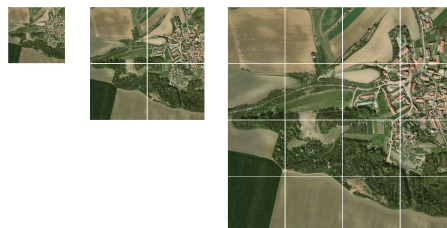
Figure 3: Part of the textures data pyramid which is created similarly like the elevation data pyramid.
