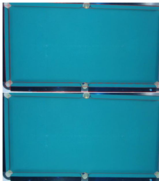
Figure 3. Top, detected lines and in the bottom final automatic table boundaries extraction.
