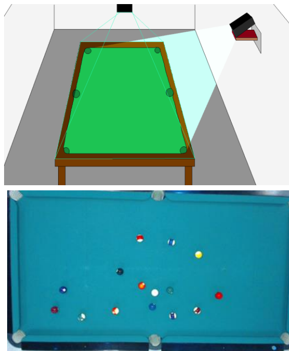
Figure 1. In the top the system layout, camera and projector position in relation to the pool table. In the bottom, the one acquired image (frame).
