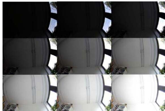
Figure 2. Nine images captured with a fish-eye lens at different exposure levels
