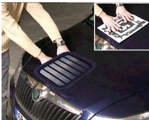
Figure 6: Marker occlusion. The marker is approx. 2 m distant from the camera.
