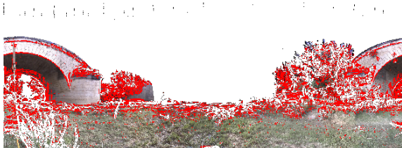
Figure 8: Results for the real scene. Points detected as unstructured are marked in red. Neighbourhood window size: 9.
