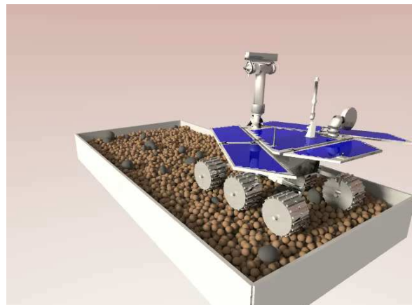
Figure 1: Simulation of a complex multi-rigid-body mechanism with contacts and joints.
