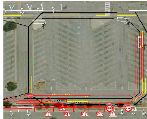
Figure 9: A qualification test of the DARPA Urban Challenge was recreated with vIsage, other dynamic vehicles (white rectangles) were added. The concrete barriers (red and white) were recreated using their original positions. The red triangles indicate that they were identified as obstacles on our vehicle's driving lane.
