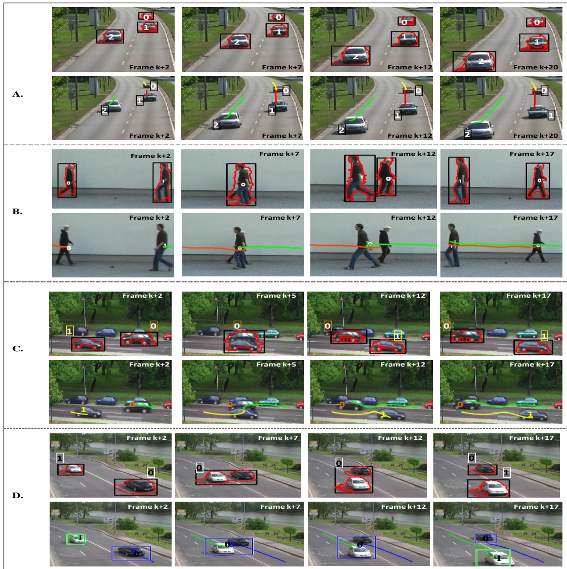
Figure 3. Analysis results of moving cars with motion trajectories (trajectories are associated with Index Numbers). In A, the car are tracked through the indexes and shows the tracking in normal case. In B, two moving people are fully occluded in the frame k+7. It is observed that the objects are tracked during merge and split. In C, two moving cars with same color are traced after confusion because we are not relying on single feature. So, we are able to maintain the identities of objects and assist Tracker. In D, the merge occurs due to shadows but the ACAP assisted Kalman tracker is able to track both the cars during the complex situations.
