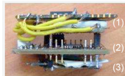
Figure 4. WiMoCa Sensing Node structure: (1) Communication – Bluetooth transceiver; (2) MSC/Sensors – ATMega8 & Triaxial Accelerometer; (3) Power Supply
