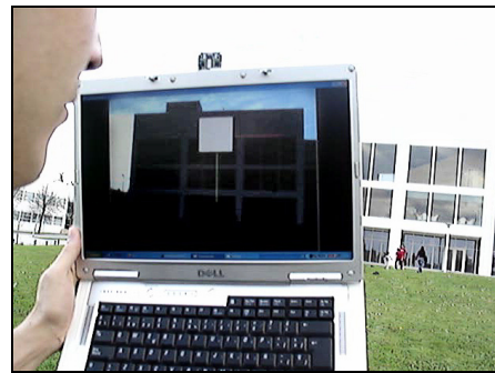
Figure 11: Outdoor Tracking of a building facade.
