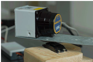
Figure: 3D scanner (rotating 2D Hokuyo laser range finder)
