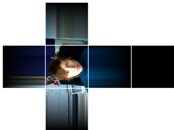
Figure 3. The environment cube map is built from the camera's input through cropping, the repetition of the final rows and columns, and feathering.
