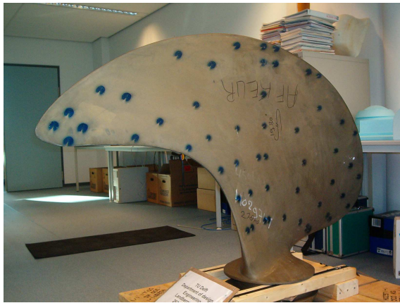
Figure 1. Example of a propeller blade. The marks on the surface indicate the locations of the verification measurements.
