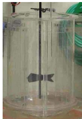
Figure 1: Stir Tank (Courtesy Dow Chemicals)
