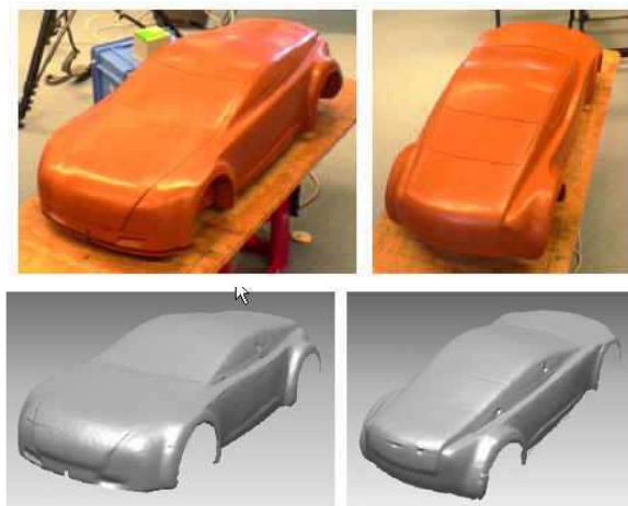
Figure 8 A 1:5 automotive model (top) was fully automatically registered and merged into a surface model (bottom).
