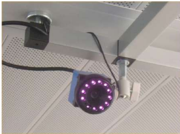
Figure 2: Camera and (optional) infrared light beamer
