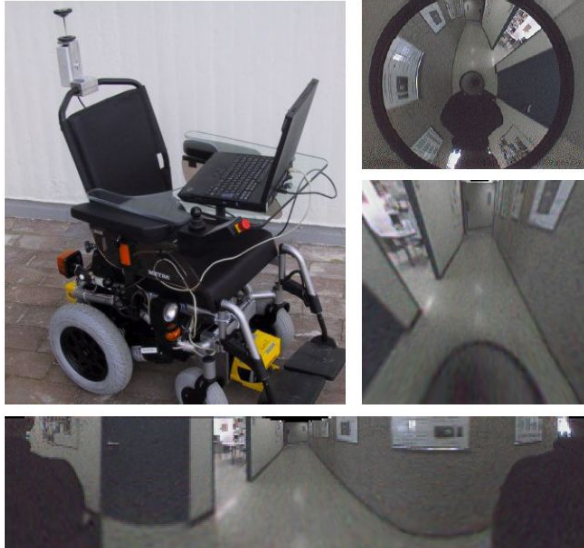
Figure 8: The autonomous wheelchair. The camera image (top-right) showing the omnidirectional view can be unwrapped into both perspective views (center-right) and into the panoramic view (bottom).
