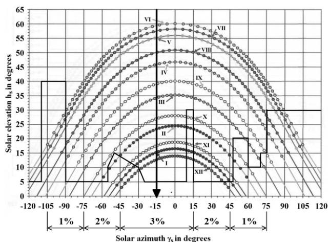
Fig. 1. Shading diagram and weight of shadowing points for 53°N [1]
