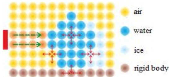
Figure 4. Heat transfer between particles of different mediums
