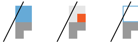
Figure 8: On the left, a view ray hits the blue octree node which should be refined. In the middle, the children of the blue node are highlighted in red. As all children are invisible, we mark the blue node for occlusion rendering only in the next frame.
