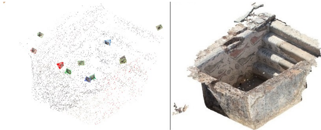
Figure 3: Sparse (left) and dense (right) point cloud of the quadrangular Pool
