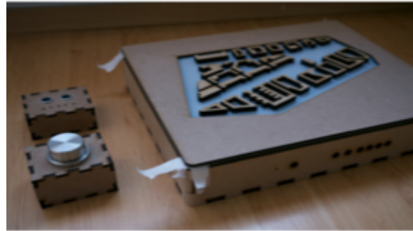
Fig 4. Experience prototype with scale model and integrated LCD display, controllers (ultrasonic sensor and rotary dial) on the left.
