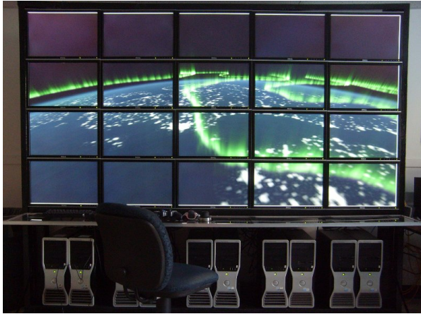
Figure 12: Interactive aurora rendering on a powerwall cluster with ten GPUs and twenty screens at 29fps.
