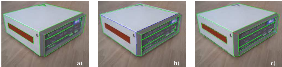
Figure 9: Rendering of augmented camera images at different steps of the recognition process. Detected and vectorized edges of the camera images are shown in a). A hypothesis (blue) generated by the approach of Dhome [7] and model's feature lines are seen in b). A finally checked and improved solution—based on Lowe [11]—is displayed in c). The red line segment could not be matched in the camera image.
