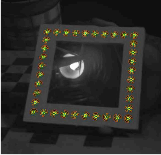
Figure 3: The tracking process: We find the rotationally invariant features (correctly identified features are shown in orange) and track them through the video sequence. The features encode positions on the mirror plane. This allows us to compute a homography between mirror coordinates and image coordinates which in turn facilitates camera calibration.
