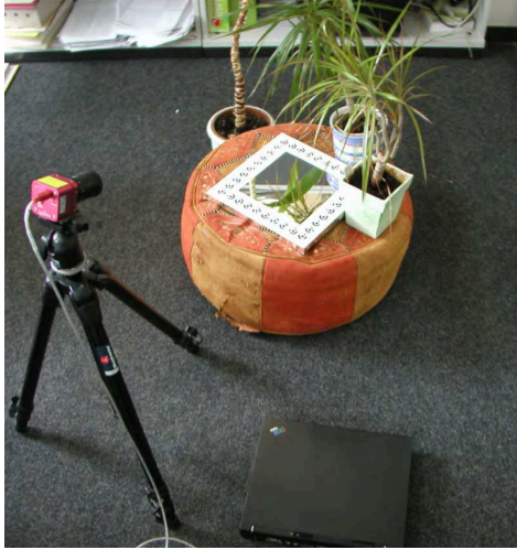
Figure 1: Our recording setup consists of a HDR video camera, an acquisition laptop and a planar optical front surface mirror with a frame of rotationally invariant binary coded patterns.
