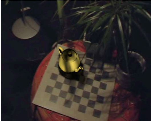
Figure 11: Real world scene with augmented teapot. The shadows of the recorded light field are faithfully rendered on the modeled geometry. Shadows cast by the teapot are generated by the recorded light source and blended with the background image.
