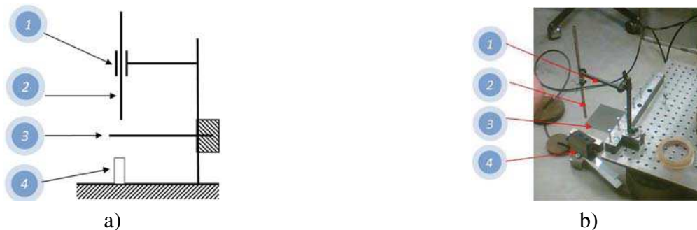
Fig. 6. Experimental measurement: a) experimental schema, b) actual photograph from measurement (1 – tube fixture, 2 – impactor guide tube, 3 – composite plate, 4 – optoNCDT laser sensor)
