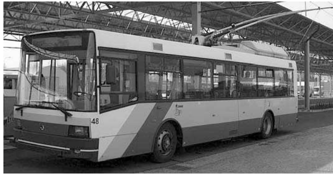
Fig. 1. The ŠKODA 21 Tr low-floor trolleybus
