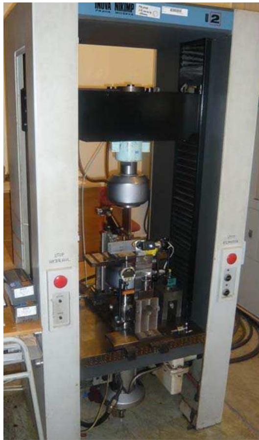
Fig. 4. The three-point bending fatigue test configuration
