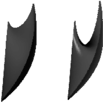
Figure 10: Symmetrical petal: (a) the top four control points pull down the curve; (b) the middle two control points on the top pull further down.
