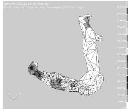
Figure 12: von-Mises average stress induced into the mandible
