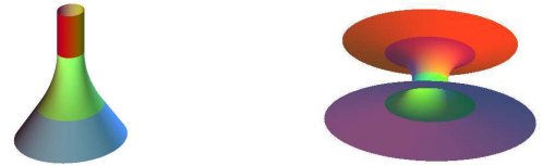
Figure 11: Left. cylinder-cone blending. Right. cone-cone blending
