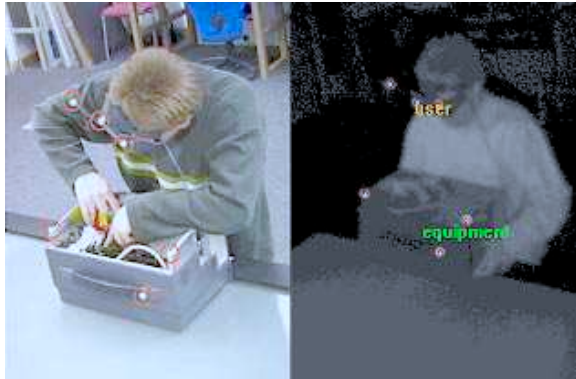
Figure 4: View on tracked person and object from a normal camera and the infrared camera
