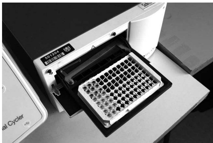
Picture 4. The device for measuring the absorbance of the resulting reaction of the microplates – ELISA reader VERSAmax™ (Molecular Devices).
