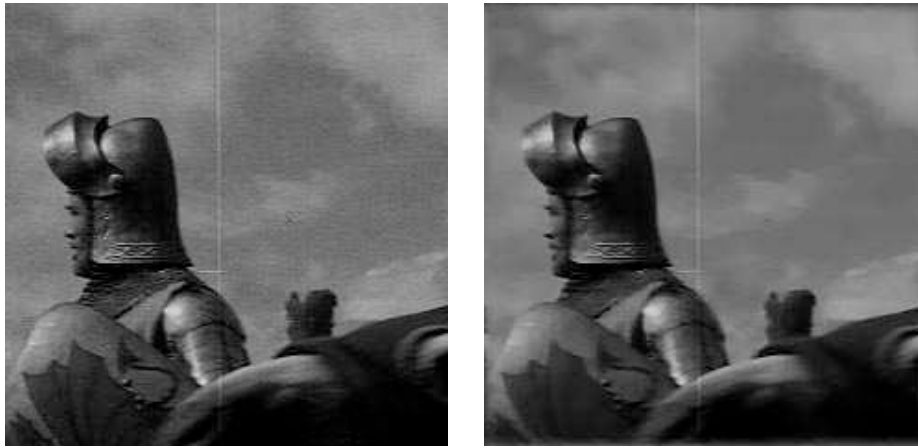
Figure 5: Knight sequence: left) 35 th noisy frame; right) 35 th restored frame. Notice that the image has been only denoised and then it is still affected by other kinds of degradation like scratches.
