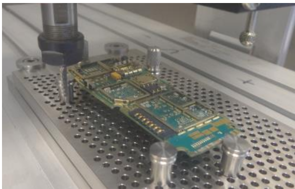
Fig. 3: Photo of the PCB holder with milling tool
