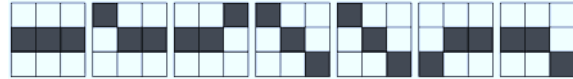
Figure 2. Gradient masks for vertical-like oriented gradient-based segmentation step (gray box means g(i,j) > g_t ). Oriented gradient matrix obtained for current pixel is compared with each gradient mask. When template is matched, current pixel is added to the foreground.
