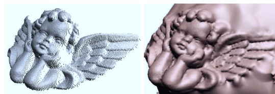
Figure 1: Example of surface reconstruction from unorganized points.
