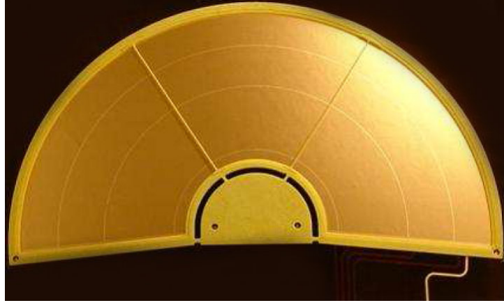
(b) The T2 GEM foil glued to the support.
