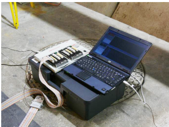
(a) Portable computer with a cable tester.
