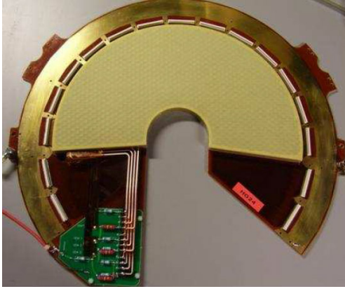
(a) T2 Gas Electron Multiplier With the high voltage divider without frond-end electronics
