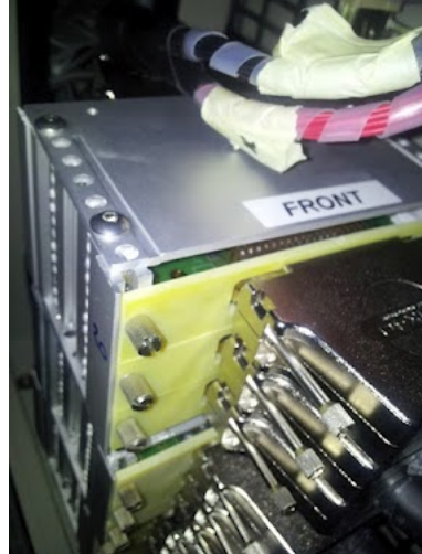
Figure 3.20: Mechanical box (repeater box) for the repeaters. Each box carries three repeaters. The box provides sufficient protection against the mechanical stress created by the cabling.
