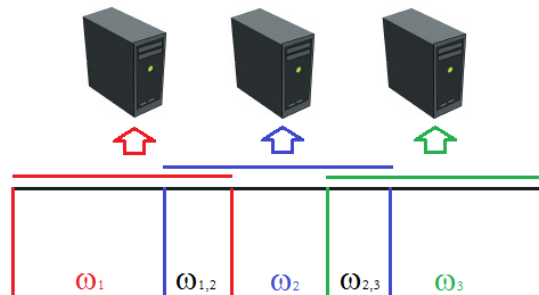
Figure 1: Partition of computational domain \Omega into three overlapping subdomains \omega_1 , \omega_2 and \omega_3 with overlaps \omega_{1,2} and \omega_{2,3} .
