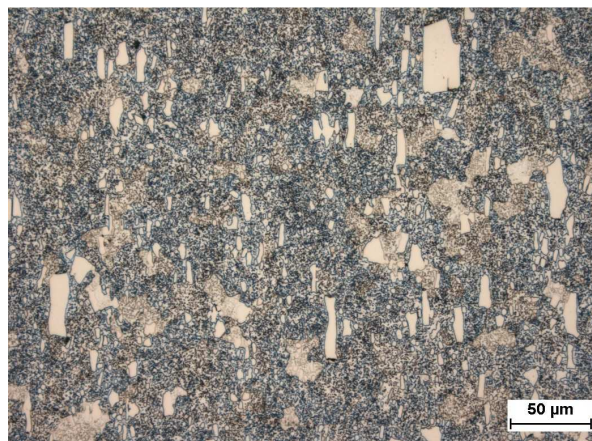
Fig. 2: Basic structure of analyzed material, light microscope, Nital etching
