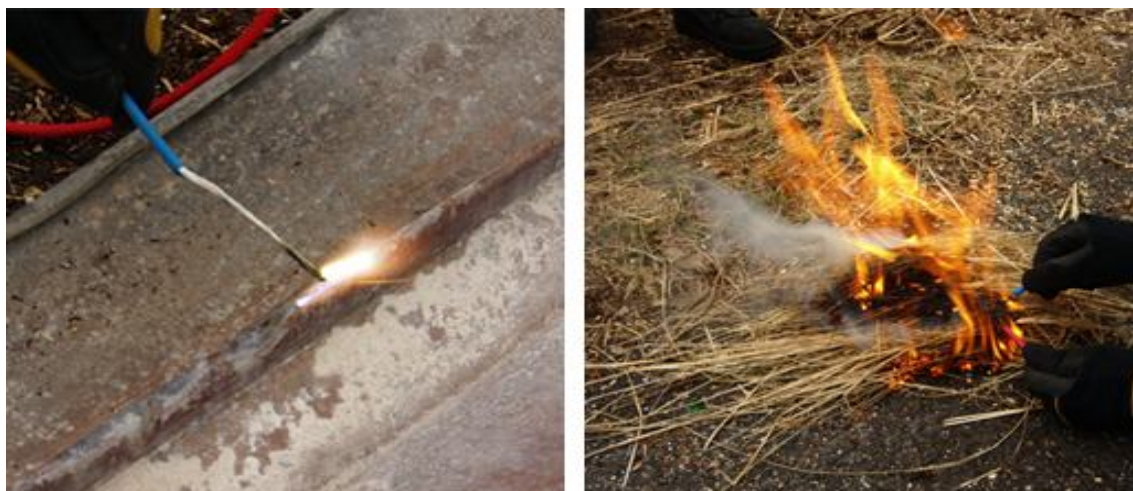
Figure 2 – PV panels powered DC arch (0,75 A) and fire initiation.
