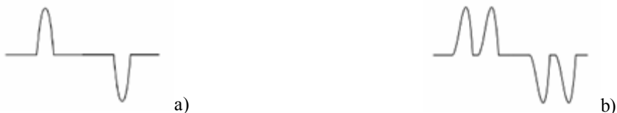
Figure 5 – Non-harmonic current waveforms for devices containing a) one-phase rectifier and smoothing capacitor, b) six-pulse rectifier and smoothing capacitor
