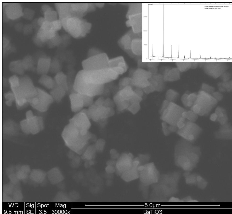
Figure 1 – Crystals of barium titanate prepared in hydroxide melt
