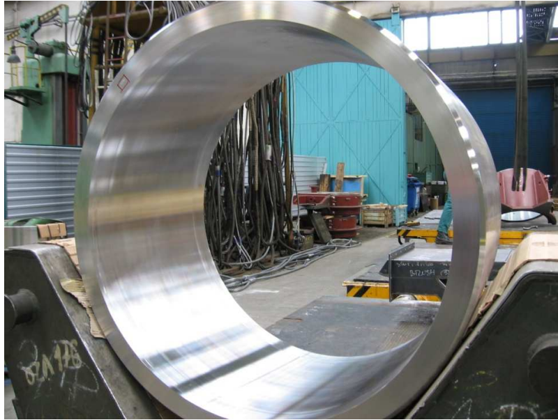
Figure 1 – 200MW turbo-generator shrink-ring
