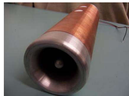
Fig.1: New design of gerdien condenser ( M=0,75 \text{ dm}^3 , v=0,8 \text{ ms}^{-1} , I_{leak}=0,05 \text{ pA @ } 150\text{V} )
