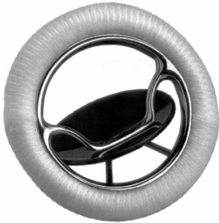
Figure 2 – Photograph of BSCC prosthetic heart valve. Tilting disc is held in place between fixed inlet strut (foreground) and welded smaller outlet strut (background). Whiter outer material is sewing ring, [4]
