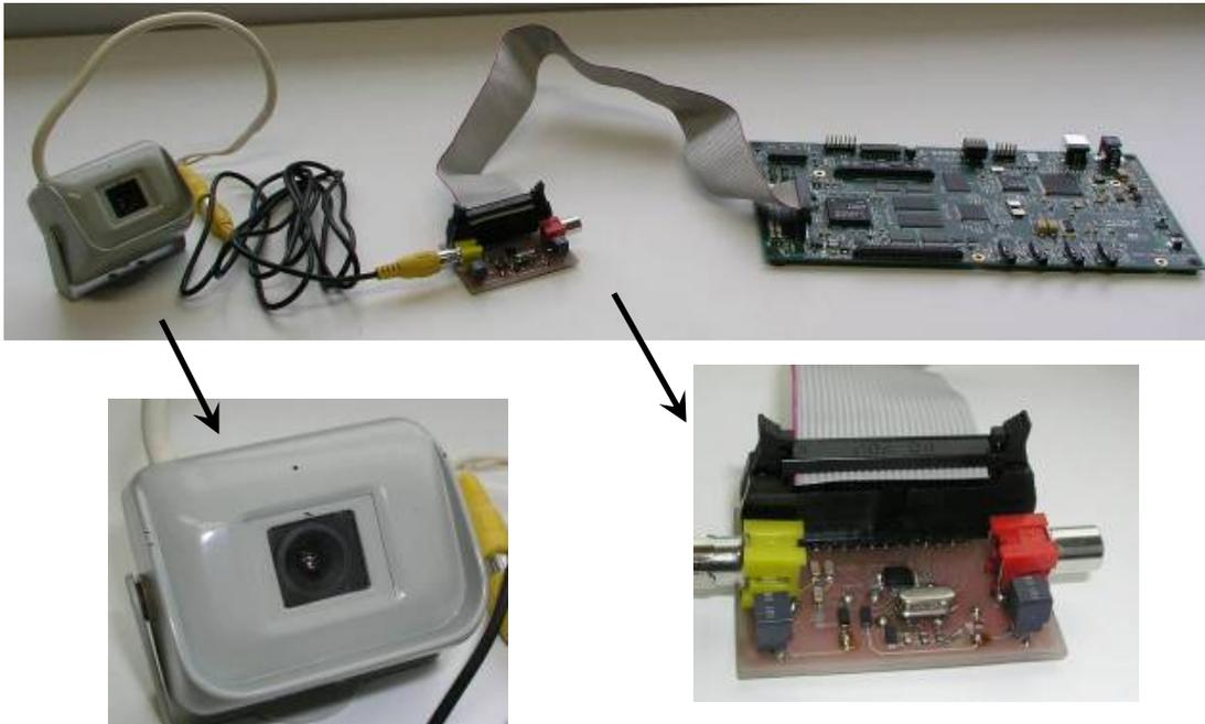
Fig. 3 Basic parts of the passive optical locator with limited range
