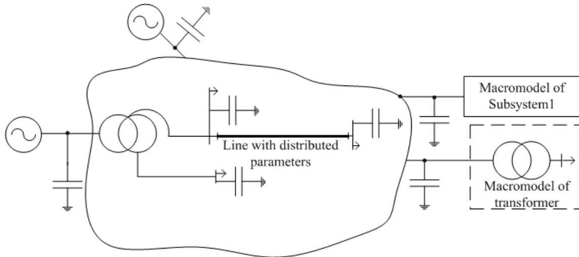
Fig. 2. Generalized scheme of electric system for transient research on the basis of mathematical models and macromodels
