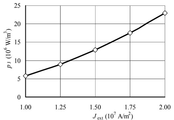
Fig. 7: Dependence of specific Joule losses  $p_j$  in dilatation element **2** on the field current density  $J_{ext}$  in field coil **1** ( $f = 50$  Hz)
