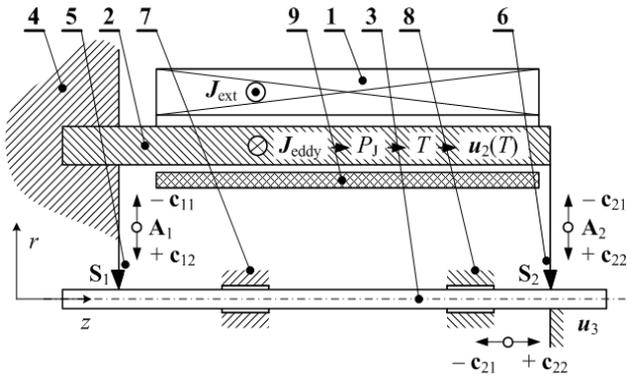
Fig. 1. Schematic arrangement of the controllable thermoelastic actuator:
