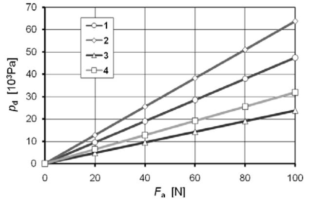
Fig. 15: Dependence of pressure  $p_d$  in the conical surface of clutch  $\mathbf{S}_2$  on force  $F_a$  generated by actuator  $\mathbf{A}_2$
