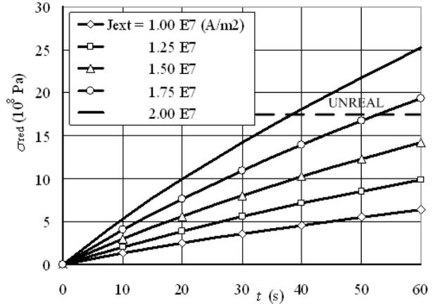
Fig. 10: Distribution of the reduced stress  $\sigma_{\text{red}}$  (according to the van Mises hypothesis) of the dilatation element 2 in time  $t$  as a function of field current density  $J_{\text{ext}}$  (for  $f = 50$  Hz)
