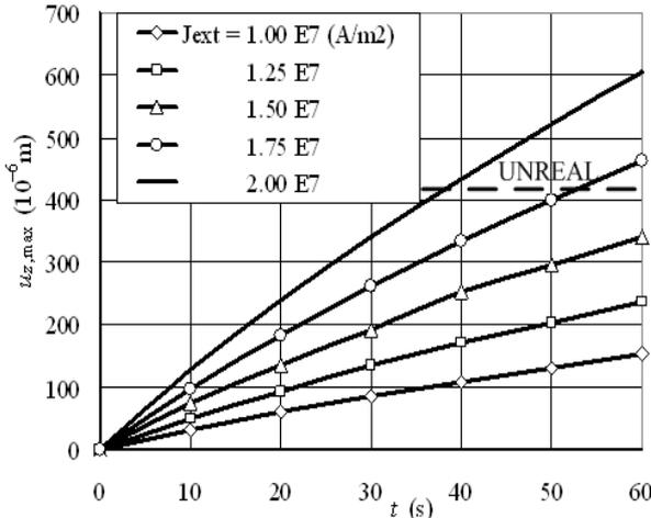
Fig. 9: Distribution of maximum thermoelastic displacement  $u_{z,\text{max}}$  of the dilatation element 2 in time  $t$  as a function of field current density  $J_{\text{ext}}$  (for  $f = 50$  Hz)
