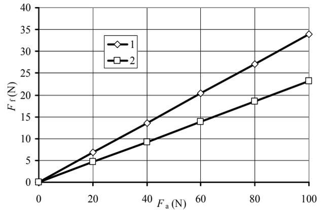
Fig. 16: Dependence of the friction force  $F_f$  in clutch  $\mathbf{S}_1$  on the axial force  $F_a$  generated by actuator  $\mathbf{A}_1$
