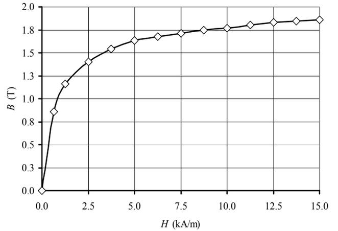
Fig. 5: Dependence  $B(H)$  of steel CSN 12 040 (see [4])
