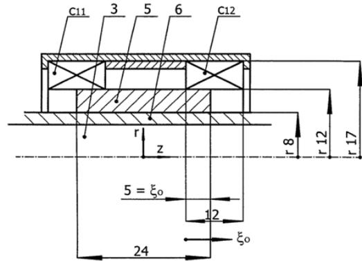
Fig. 3a: Arrangement of electromagnetic actuator  $A_1$ :
