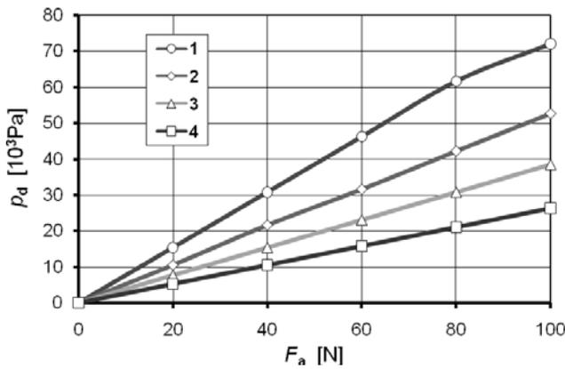
Fig. 14: Dependence of pressure  $p_d$  in the conical surface of clutch  $\mathbf{S}_1$  on force  $F_a$  generated by actuator  $\mathbf{A}_1$
