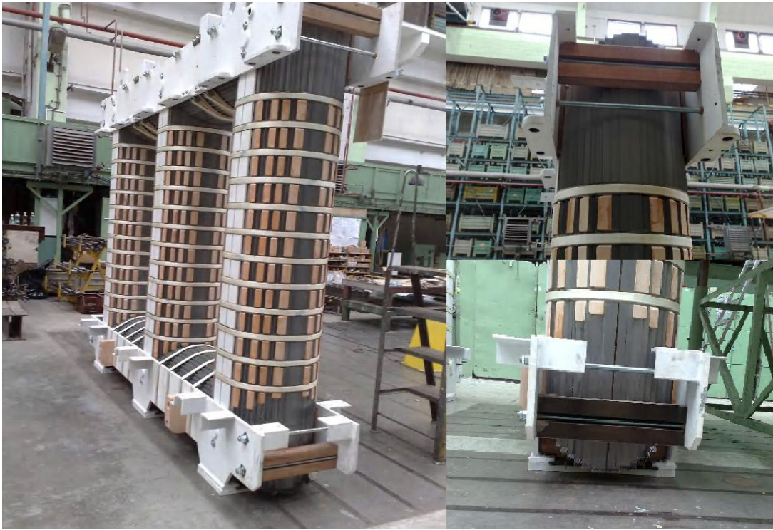
Fig. 4. Magnetic circuit of transformer and frame construction
